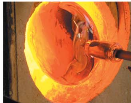
Photo Credit: Michael Sider, 2005. A piece being re-heated at the "glory hole" in the hot shop at New-Small & Sterling Studio. The piece is from the Marine Reliquary series by David New-Small. The "glory hole" is a natural gas-powered furnace which operates at about 1200° C and is used to re-heat glass work in progress, to keep it malleable as the "gaffer" (master glassblower) shapes the piece.
